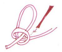
**Step 6: Testing, testing.** After you've gotten it through the back of the harp, pull up hard on the string to see if you have a good knot that's holding the anchor. If you hear a little "clink" inside the sound box., your anchor has escaped. You're not alone; the bases of all my harps are small graveyards of anchors that refused to stay put. Just wiggle another anchor into the existing knot and you're back on your way.
