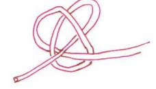
Tighten it partway. Insert your anchor, then tighten the knot again as much as you can. Make that knot really grab the anchor, so it stays put when you let go.
